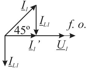
$$I_l' = \frac{\underline{U}_l}{\underline{Z}} = \frac{\underline{U}_l e^{j0^\circ}}{Z e^{j\varphi}} = \frac{230}{20\sqrt{2} e^{-j45^\circ}} = 8,13 e^{j45^\circ} A$$
