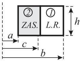
$$W_{m2} = \frac{1}{2} B_{K2} H_{K2} V_2 = \frac{1}{2} B_{K2} H_{K2} (c^2 - a^2) \pi h$$
