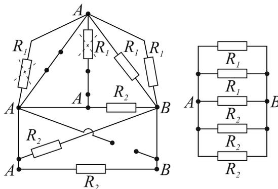
$$R_T = R_{AB} = R_1 \parallel R_1 \parallel R_2 \parallel R_2 \parallel R_2$$
