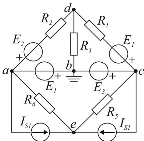
$$V_b = 0V, \quad V_a = -E_1 = -5V \quad V_c = E_3 = 13,4V$$
