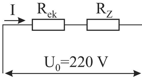
$$I = \frac{U_0}{R_{ek} + R_Z} \leq I_{max} \quad (I_{max} = 300 mA)$$
