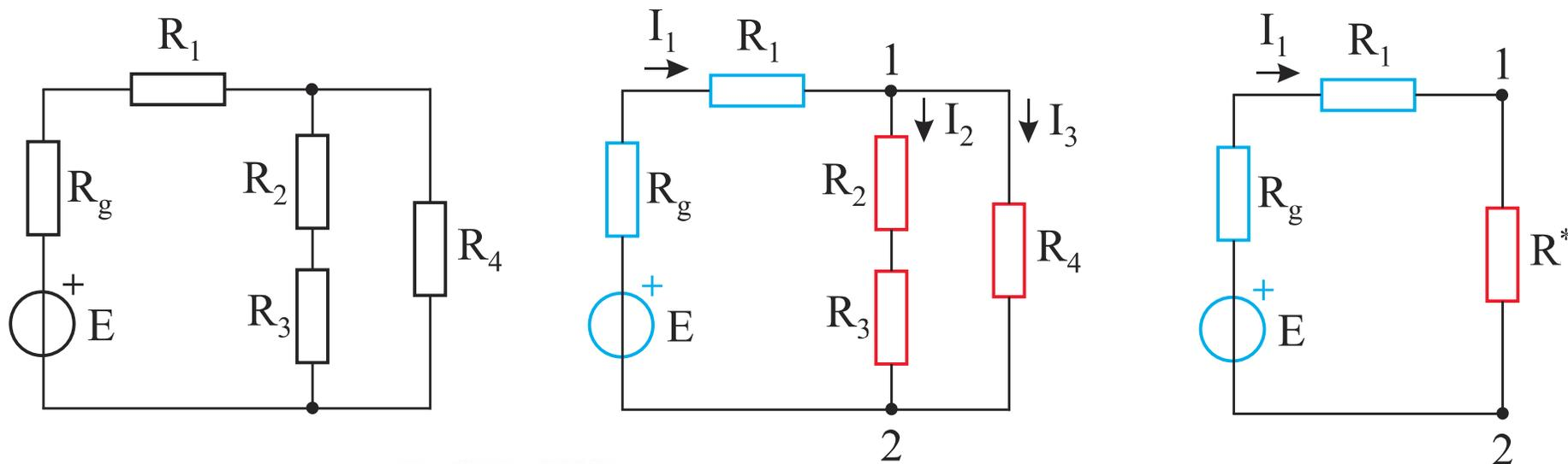
$$R^* = R_4 \parallel (R_2 + R_3) = \frac{R_4 \cdot (R_2 + R_3)}{R_4 + (R_2 + R_3)} = ?$$
