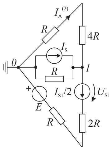
$$\begin{aligned} V_0 &= 0 \text{ V} \\ \hline V_1 & \left( \frac{1}{5R} + \frac{1}{\infty} + \frac{1}{R} + \frac{1}{3R+\infty} \right) = I_S - \frac{I_{S1}}{2} \\ \hline V_1 & \left( \frac{1}{5 \cdot 35} + \frac{1}{35} \right) = 100m - 240m & / \cdot 5 \cdot 35 \\ \hline 6V_1 & = -24,5 \quad \Rightarrow \quad V_1 = -4,08 \text{ V} \end{aligned}$$
