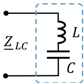
$$\underline{Z}_{LC} = \underline{Z}_L + \underline{Z}_C = 0$$
