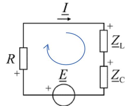
$$\text{KZ: } -\underline{E} + R\underline{I} + \underline{Z}_L\underline{I} + \underline{Z}_C\underline{I} = 0$$
