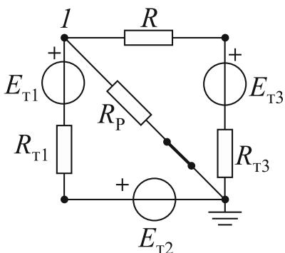
$$\left( \frac{1}{R_{T1}} + \frac{1}{R_P} + \frac{1}{R + R_{T3}} \right) V_1 = \frac{E_{T1} + E_{T2}}{R_{T1}} + \frac{E_{T3}}{R + R_{T3}}$$
