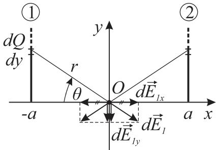
$$d\vec{E}_{1x} + d\vec{E}_{2x} = 0 \quad z \text{ bog simetrije}$$
