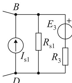
$$R_{T3} = R_{BD} = R_{s1} \parallel R_3$$
