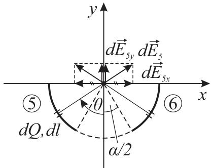
$$d\vec{E}_{5x} + d\vec{E}_{6x} = 0 \quad z \text{ bog simetrije}$$
