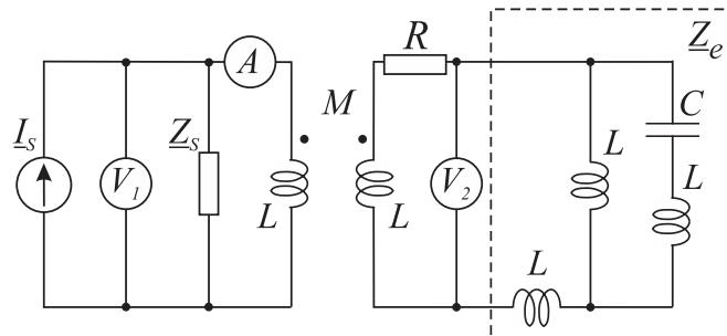
Brojni podaci su:  $I_s = (1+j) \text{ A}$ ,  $L = 20 \text{ mH}$ ,  $C = 250 \text{ nF}$ ,  $M = 10 \text{ mH}$ ,  $R = 50 \Omega$ ,  $Z_s = (50-j100) \Omega$ .
