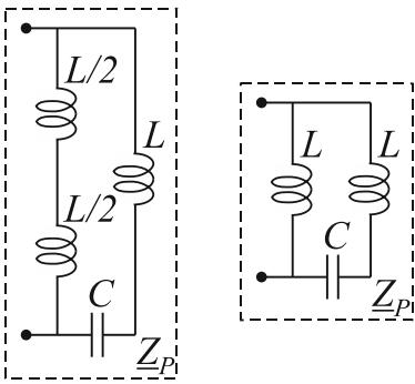
$$\underline{Z}_1 = j\omega L + \frac{1}{j\omega C} = \frac{1 - \omega^2 LC}{j\omega C}$$
