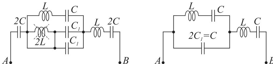
$$\underline{Z}_1 = j\omega L + \frac{1}{j\omega C} = \frac{1 - \omega^2 LC}{j\omega C}$$
