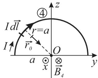
$$\vec{dB}_4 = \frac{\mu_0}{4\pi} \frac{I \vec{dl} \times \vec{r}_0}{r^2} \quad dB_4 = \frac{\mu_0}{4\pi} \frac{I dl}{a^2} \quad \sphericalangle(\vec{dl}, \vec{r}_0) = \frac{\pi}{2}$$
