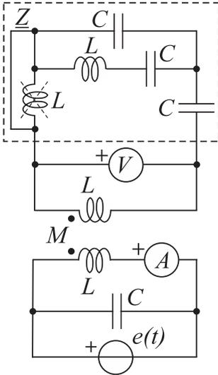
$$\underline{Z}_1 = j\omega L + \frac{1}{j\omega C} = \frac{1 - \omega^2 LC}{j\omega C}$$
