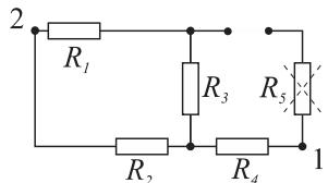
$$R_T = R_{12} = R_4 + [(R_3 + R_1) \parallel R_2] = 30 + [(10 + 10) \parallel 30] = 30 + [20 \parallel 30] = 42$$
