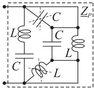
$$\underline{Z}_1 = j\omega L \parallel \frac{1}{j\omega C} = \frac{j\omega L \frac{1}{j\omega C}}{j\omega L + \frac{1}{j\omega C}} = \frac{j\omega L}{1 - \omega^2 LC}$$
