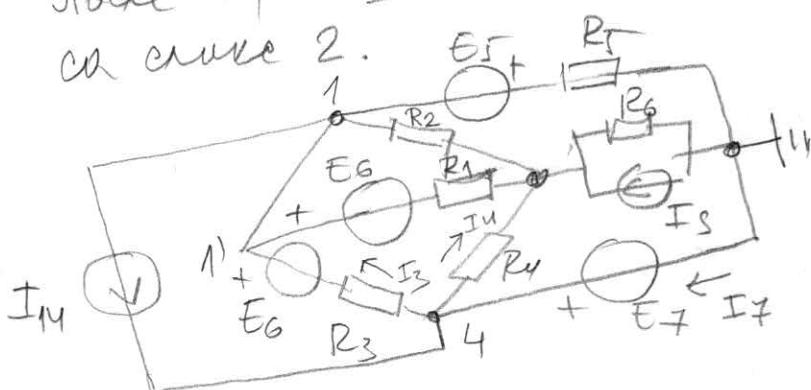
$$\begin{aligned} E_5 &= 12V & R_1 &= R_2 = 100\Omega \\ E_6 &= E_7 = 6V & R_3 &= R_5 = 300\Omega \\ I_S &= 120mA & R_4 &= R_6 = 200\Omega \end{aligned}$$
